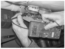
Checking pressure switch contacts.
